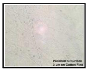
**Figure 8:** Image showing the Si surface following polishing using the Cotton Fine polishing cloth and 3 μm diamond slurry. Note the scratches on the surface which correspond to the 3 μm abrasive size with no visible pitting or mechanical damage present from the lapping process.
