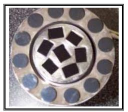
**Figure 10:** Image showing the final polished surface of the silicon die following processing. Note the specular surface and the high polish quality obtained using this process.
