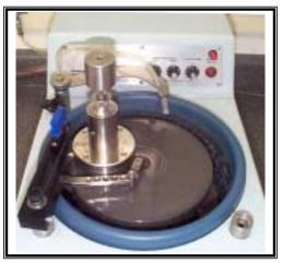
Figure 1: Setup used for lapping and polishing specimens in this experiment. A Model 920 Lapping and Polishing Machine is shown equipped with a Model 92002 Workstation and Model 155 Lapping and Polishing Fixture. The Model 155 is shown captured in the Model 92002 and is continuously rotated counter-clockwise. The lapping wheel also rotates counter-clockwise and is variable speed up to 600 rpm.
