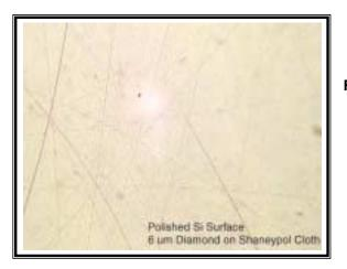
**Figure 7:** Image of the polished surface of silicon following polishing with the ShaneyPol polishing cloth and 6 μm diamond slurry. The surface of the specimen is free of mechanical damage from the lapping process and shows only surface scratches from the 6 μm abrasive media.
